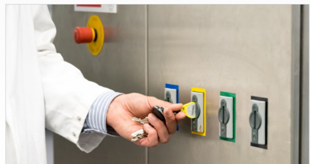
► The ingredients are unloaded at the right receiving station and into the right container via a programmed EKS chip.
