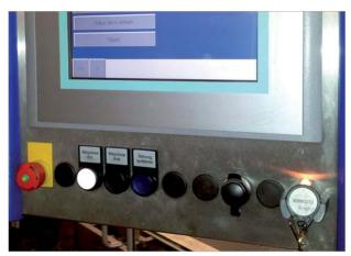
On the right side of the operating unit: the modular Electronic-Key adapter of EKS Light.
