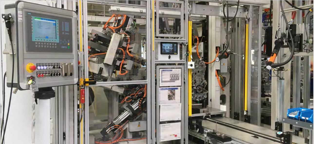
► The VW engine plant in Chemnitz uses the Electronic-Key-System EKS from EUCHNER on its assembly line for three- and four-cylinder gasoline engines. Personalized EKS Electronic-Keys for each employee ensure that only authorized users are allowed to change important process parameters on the machine control system or work in a special operating mode.
